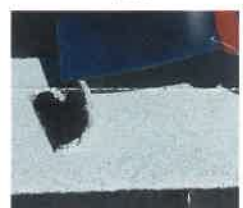
Fig. 4 Perform chisel test to verify bond. Evidence, as shown, of asphalt aggregate bonded to the underside of the lifted material indicates good adhesion.
